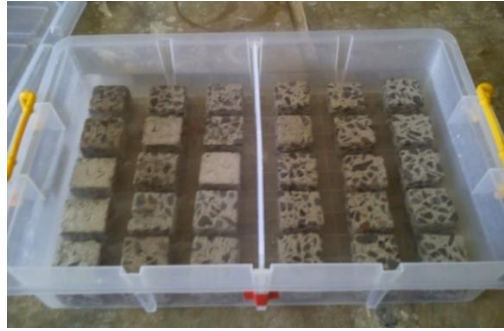
FIGURE 1. Immersion specimens in 2% and 5% sulfuric acid (H 2 SO 4 )
