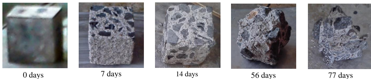
FIGURE 5. Visual condition of N30 concrete after soaking in 2% sulfuric acid ( H_2SO_4 )
