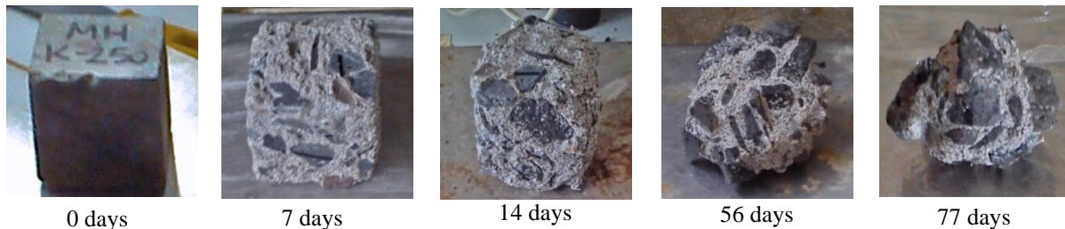
FIGURE 4. Visual condition of N20 concrete after soaking in 5% sulfuric acid ( H_2SO_4 )
